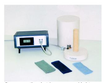
It measure the electric power provided to a heat resistance surrounded by aluminium cylinder in order to maintain a constant gap between the surface temperature of the cylinder and the cylinder environment. An electronic regulation system functioning proportionally allows for the gap to be maintained at a fixed value of 20°C.
